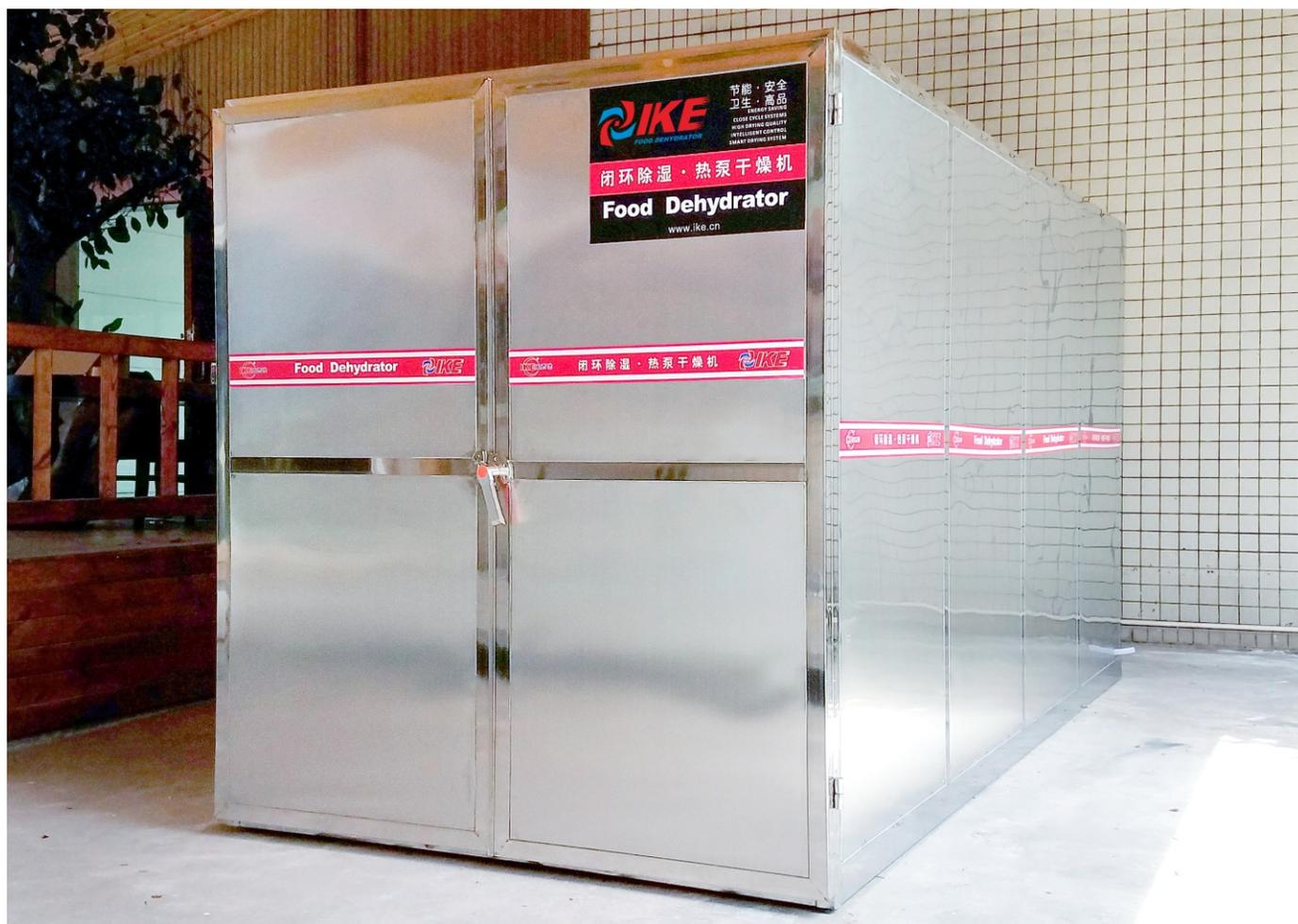
The AIO-1600 series all-in-one dehydrating system used with IKE S series drying machine, you can choose forward and reverse wind structure to achieve evenly drying by parallel airflow.
