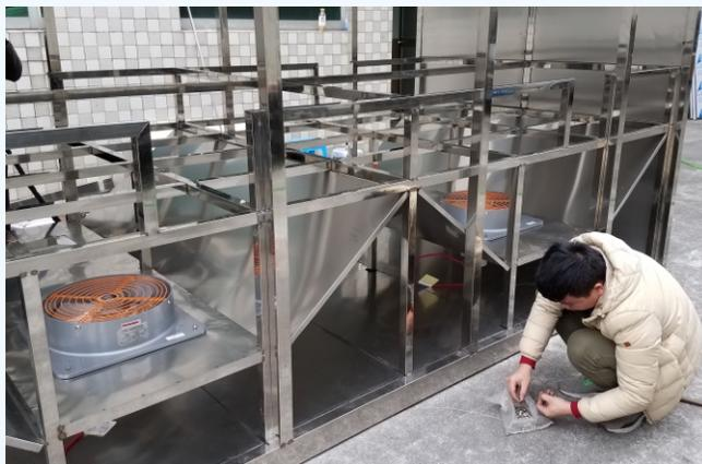
This specially structure good performance on drying the light product, such as the leaves, chives, some very easy to fly up in the drying process, we have made special mesh to cover the big tray and let them not fly and drying be better.
